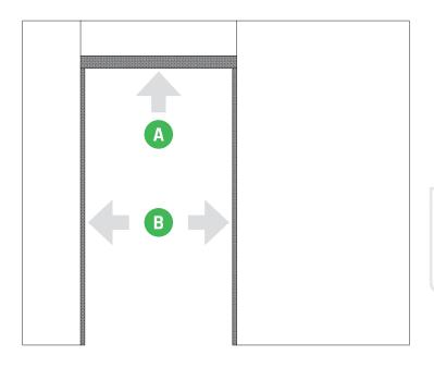
Install part A first using good quality silicon or drill and screw if preferred. measure the distance from finished floor level to the underside of  ${\bf A}$  and cut  ${\bf B}$  accordingly. secure to the frame with good quality silicon or drill and screw if preferred.
