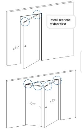
Adjust door height to be 7 mm above the floor and lock into position with by tightening lock nut
