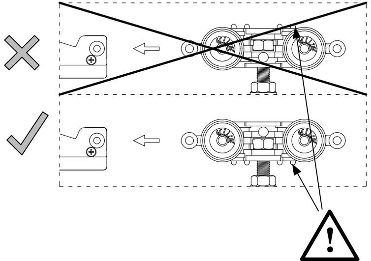
Connect the BIAS-DS mechanism to one of the rollers using the connection screw
