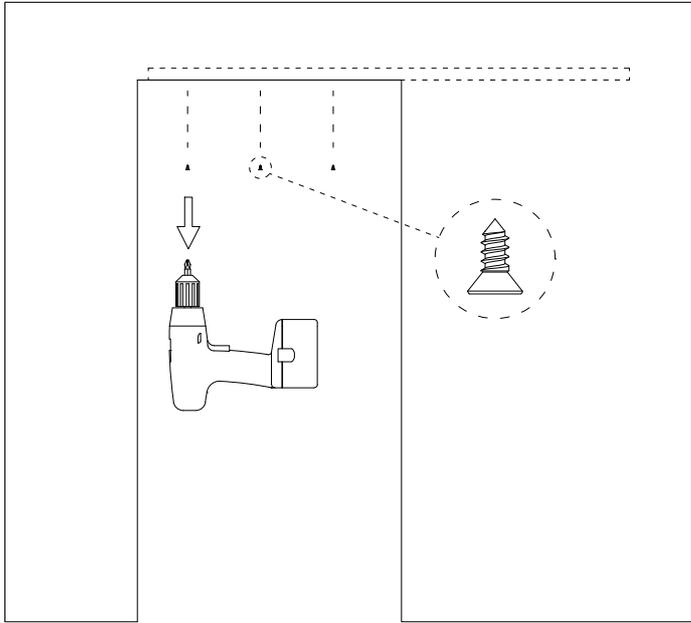
Remove track from the pocket unit by removing the small screws holding the track to the header across the opening. Slide the track to one side and it will drop out.
