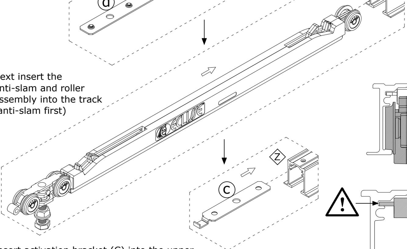
Insert activation bracket (C) into the upper slot of the track as per above drawing. NOTE: Take care to insert the bracket in the correct orientation as shown.
