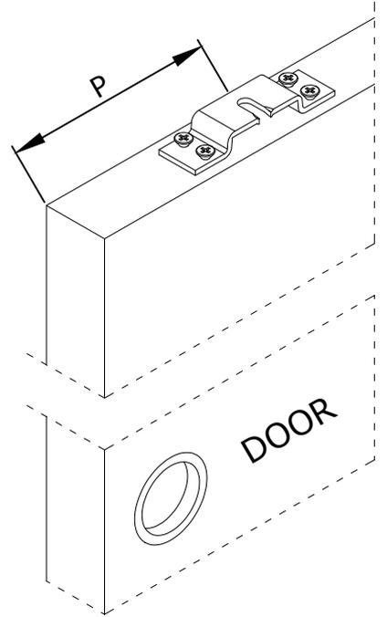
Set activation bracket (C) in place. Pre-drill the holes for ease and follow up with the screws (E)
