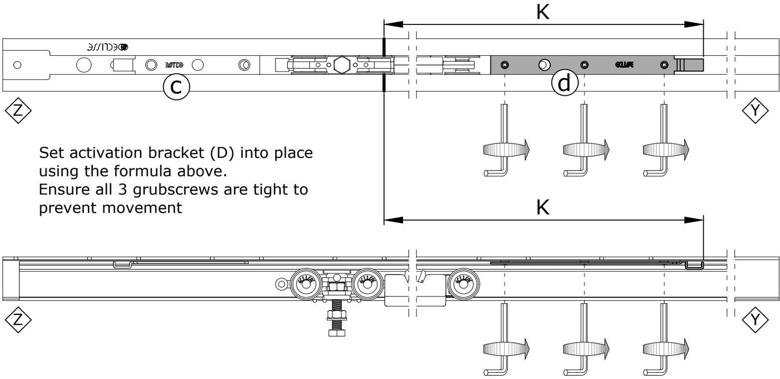
Set activation bracket (D) into place using the formula above. Ensure all 3 grub screws are tight to prevent movement
