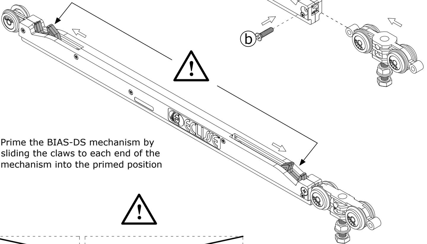
Prime the BIAS-DS mechanism by sliding the claws to each end of the mechanism into the primed position
