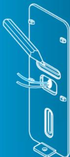
**Step 1:** Use the wall mount plate as a guide to mark the mounting holes on the surface.
